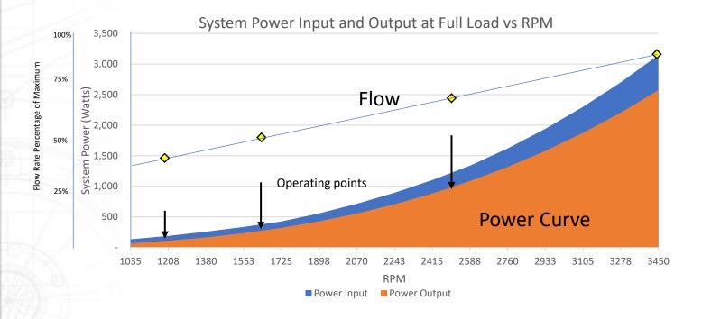
3.45HP variable speed pump motor and control power required at three operating speeds. Input power ranges from over 3000 watts at 3450 rpm to a low of less than 150 at 1200 rpm.
